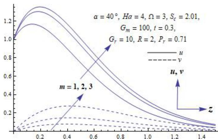
Figure 3. Primary and secondary velocity profile for different values of  $m$
