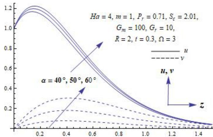
Figure 1. Primary and secondary velocity profile for different values of  $\alpha$
