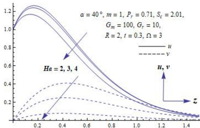
Figure 2. Primary and secondary velocity profile for different values of  $Ha$
