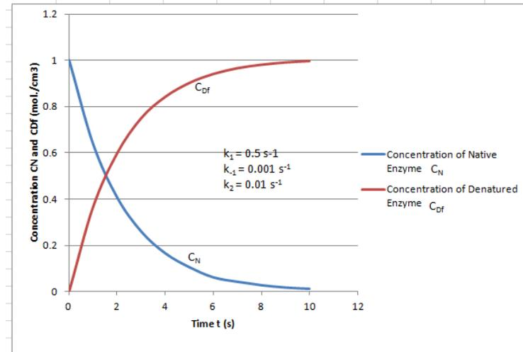
**Figure 1.** Concentration  $C_N$  and  $C_{DF}$  ( $\text{mol}/\text{cm}^3$ ) vs.time  $t$  at  $k_1 = 0.5/\text{s}$ ,  $k_{-1} = 0.001/\text{s}$  and  $k_2 = 0.01/\text{s}$
