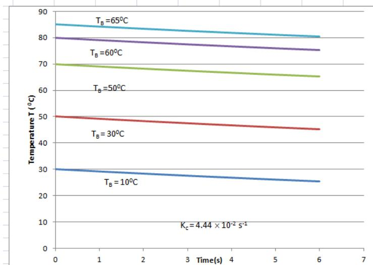
Figure 4. Temperature T vs. time t at various bath temperatures, where  $k_c = 4.44 \times 10^{-2}/s$
