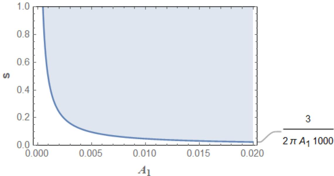
**Figure 5.** Lower bound on scaling factor  $s$  for the stability of the equilibrium point  $L_1(p_1, 0, 0)$  when  $\rho_1 = 1000 \text{ Kg/m}^3$
