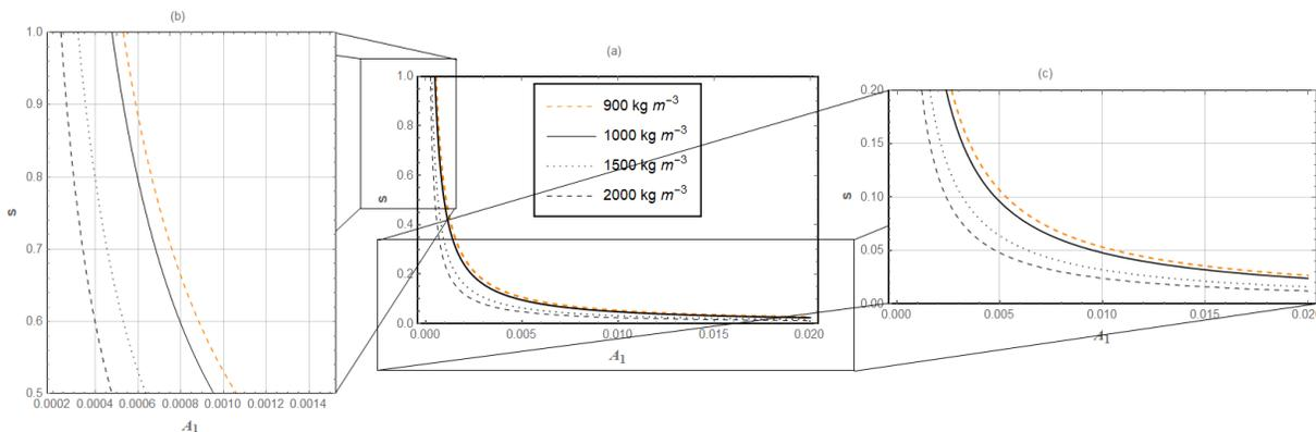
**Figure 6.** (a) Lower bound on scaling factor  $s$  for the stability of the equilibrium point  $L_1(p_1, 0, 0)$  when  $\rho_1 = 900 \text{ Kg/m}^3$ ,  $1000 \text{ Kg/m}^3$ ,  $1500 \text{ Kg/m}^3$ ,  $2000 \text{ Kg/m}^3$  (b) Show the zoomed portion of the upper part of graph (a) and (c) show the zoomed portion of the lower part of the graph (a)
