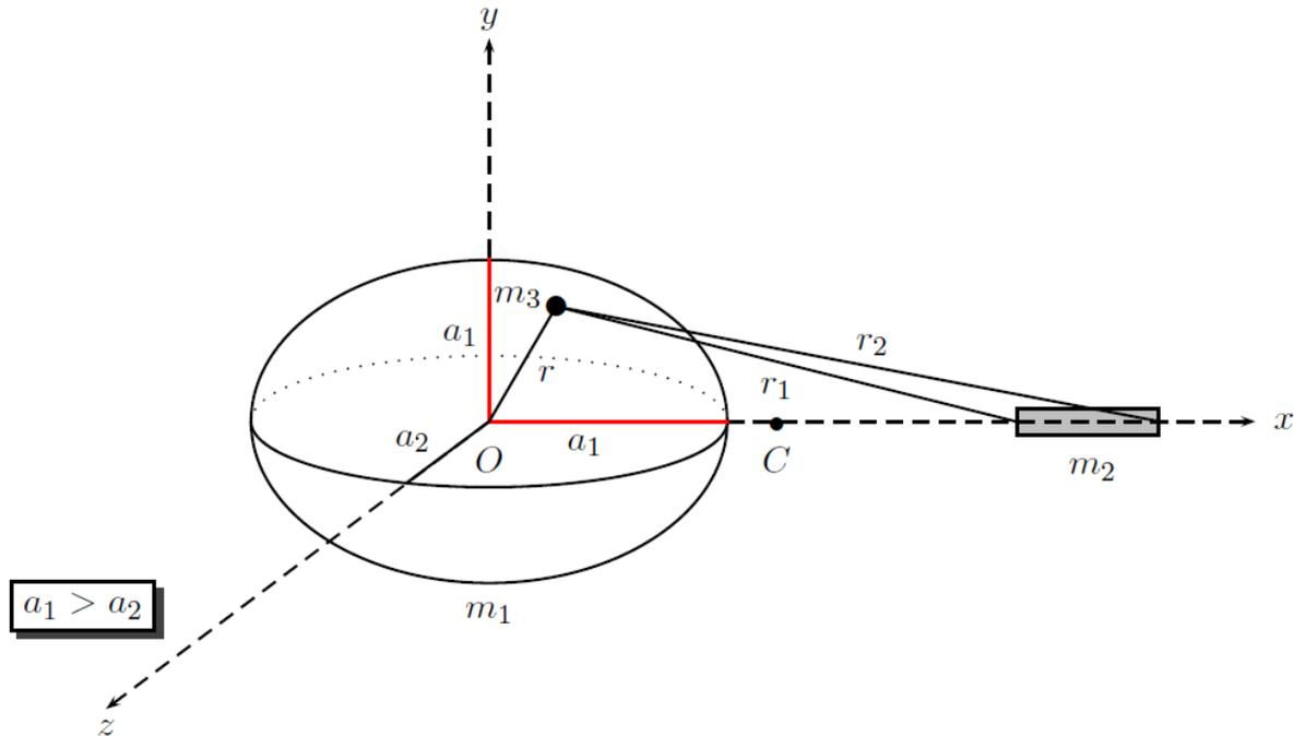
**Figure 1.** Geometric configuration of finite straight segment model of Robe's problem with an oblate body
