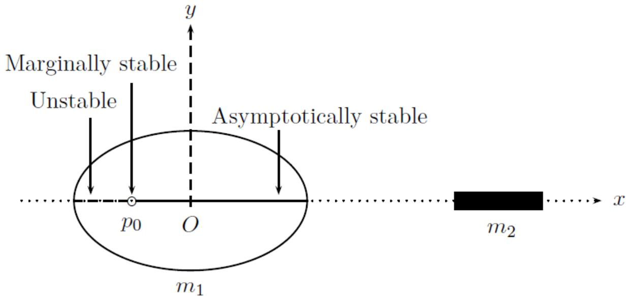
Figure 2. Bifurcation diagram for stability (in direction parallel to z-axis) of the equilibrium point  $L_1(p_1, 0, 0)$
