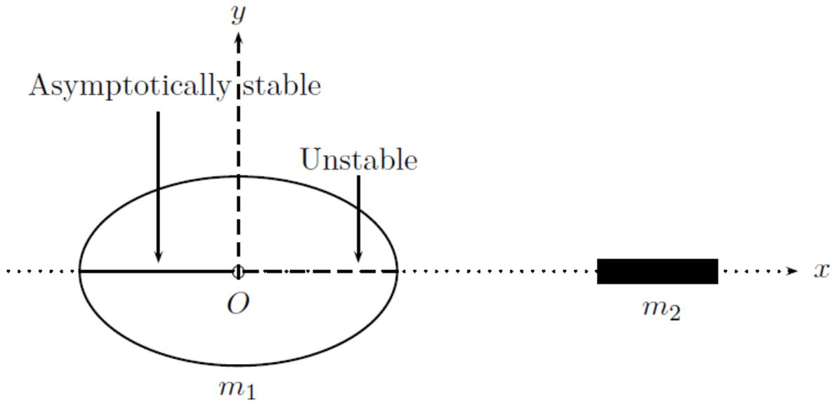
Figure 3. Bifurcation diagram for stability (in direction parallel to  $xy$ -plane) of the equilibrium point  $L_1(p_1, 0, 0)$
