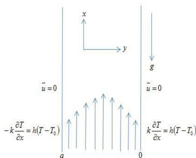
**Figure 1.** Geometry of the flow
