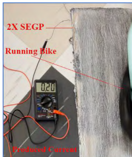
Fig. 7.13 Current Testing on the Prototype of SEGP 2X .
