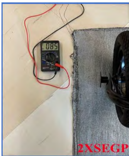
Fig. 7.14 Voltage Testing on the Prototype of SEGP 2X .
