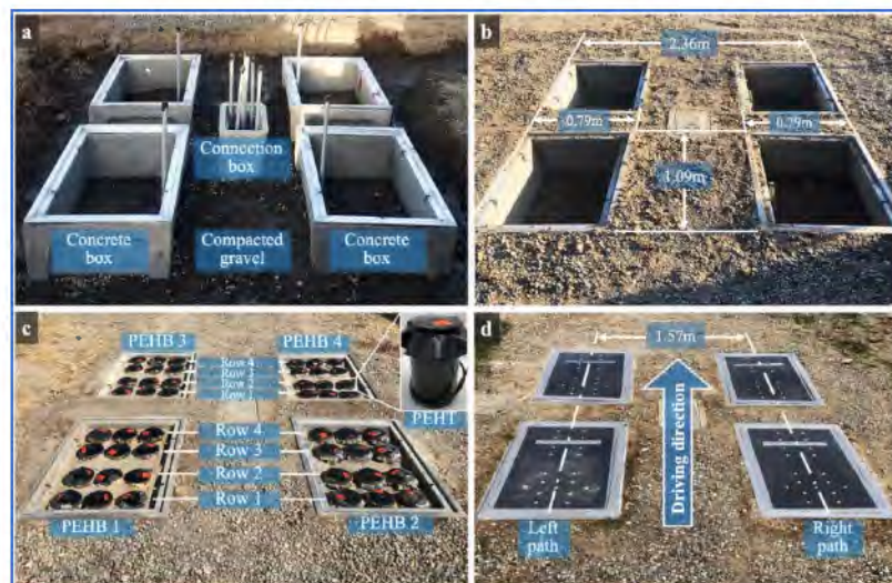
Fig. 2.13 PEHS on Road Test [71].
