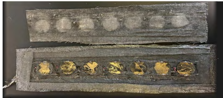
Fig. 5.18 Destructive Test and Failure Analysis on the SEGP 1X .
