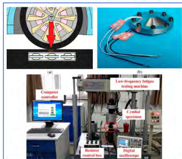
Fig. 2.9 N. Zabihi et al. development in cymbal harvesters [67].
