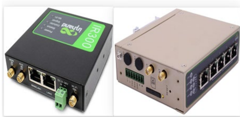
Fig. 107 In-Hand cellular modems (left). Wi-fi Switch (right) [191].
