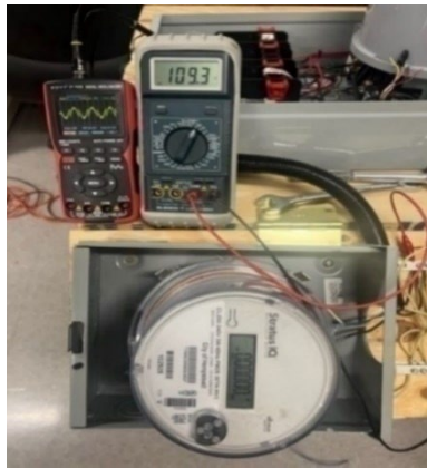
Fig. 76 Prototype Modified Sinewave and Measurements [151].
